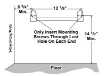
Figure 7 - Mounting Bracket Clearances
